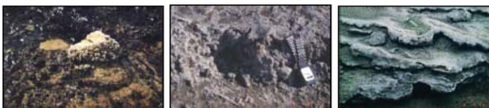
Figure 10. Uraniferous salt crusts formed well outside of tailings dams.
